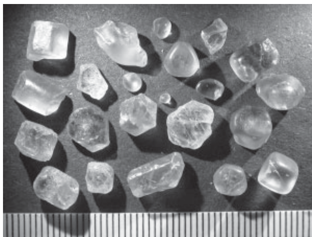
Figure 5. Sapphires from Dry Cottonwood Creek selected to show variety of shapes and surfaces typical of sapphires from this locality. Forms shown are hexagonal tablets, hexagonal prisms, irregular smooth surfaces, fractured grain, and small, almost spherical grains, many with straight grooves. Scale is in millimeters.
