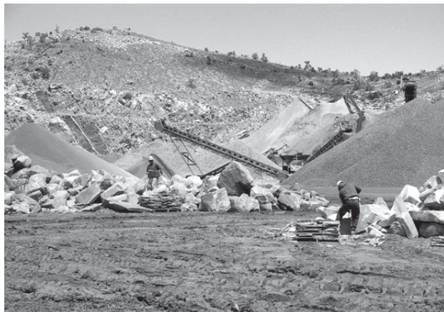
Figure 10. Hand splitting flagstone at Las Vegas Rock's Rainbow Quarries, Clark County.
