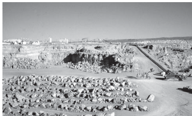
Figure 13. Gypsite beds at the PABCO gypsum mine, Clark County. PABCO’s wallboard plant is in the background.
