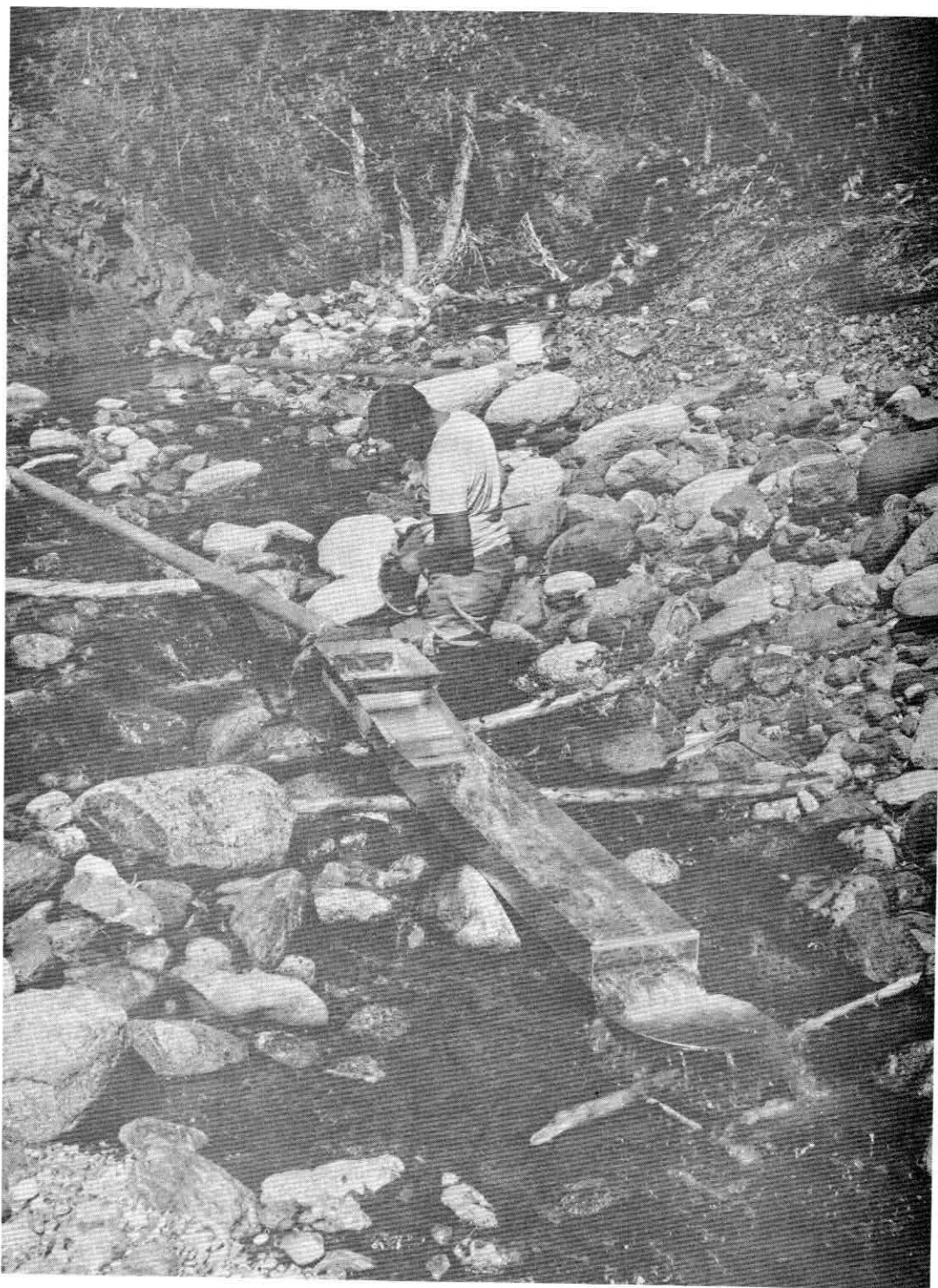
FIGURE 5. - Lightweight Sluicebox in Action. Unit made of aluminum has screen box at the head end, riffle section in the middle, and expanded metal over burlap at the foot. The gold pan would normally be omitted, but is included here to check for losses.
