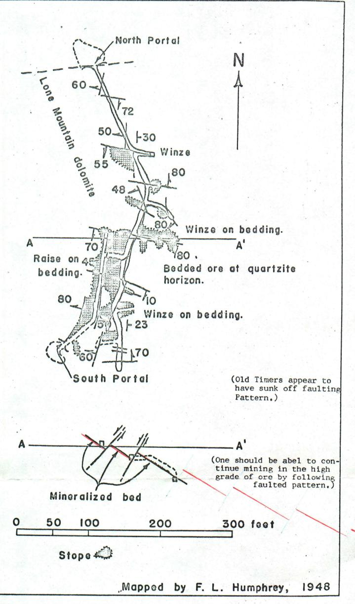
FIGURE 22. Geologic map and section of the Fay mine.
