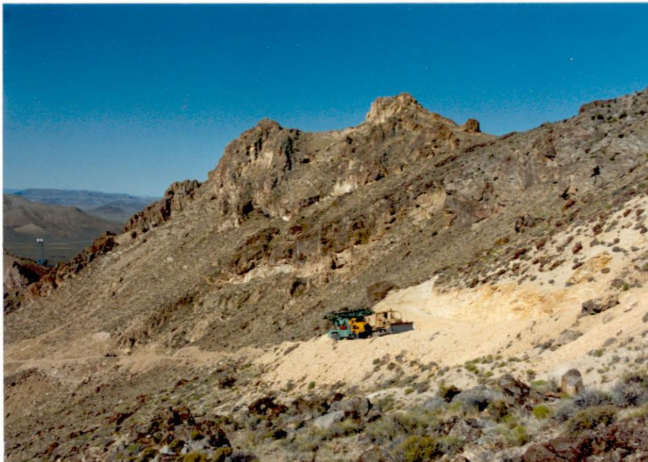
Figure 5 - Photograph of a slide block of Devonian Dolomite (gray cliffy area in center of picture). Argillized tuff of Williams Ridge and Morey Peak above and below. Dolomite above drilling is silicified and is Tuxedo Zone. Pad for SL-88-2 just behind dozer.
