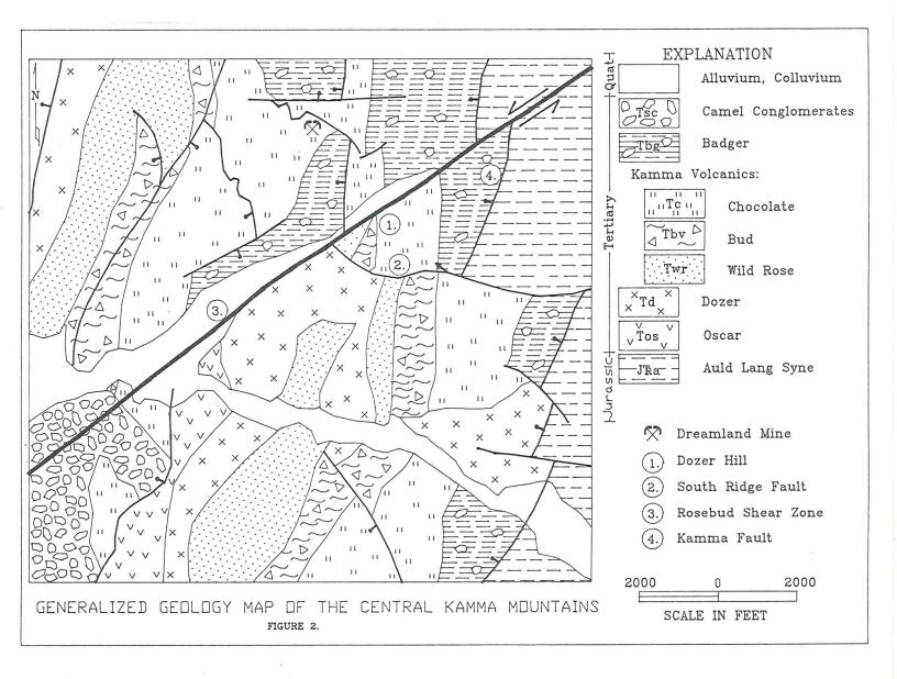
northwest, and has about 5000' of apparent left lateral displacement. Part of the left lateral movement on the eastern side of the range is taken up by the South Ridge fault, which strikes east-west and dips 25° to 45° to the north.
