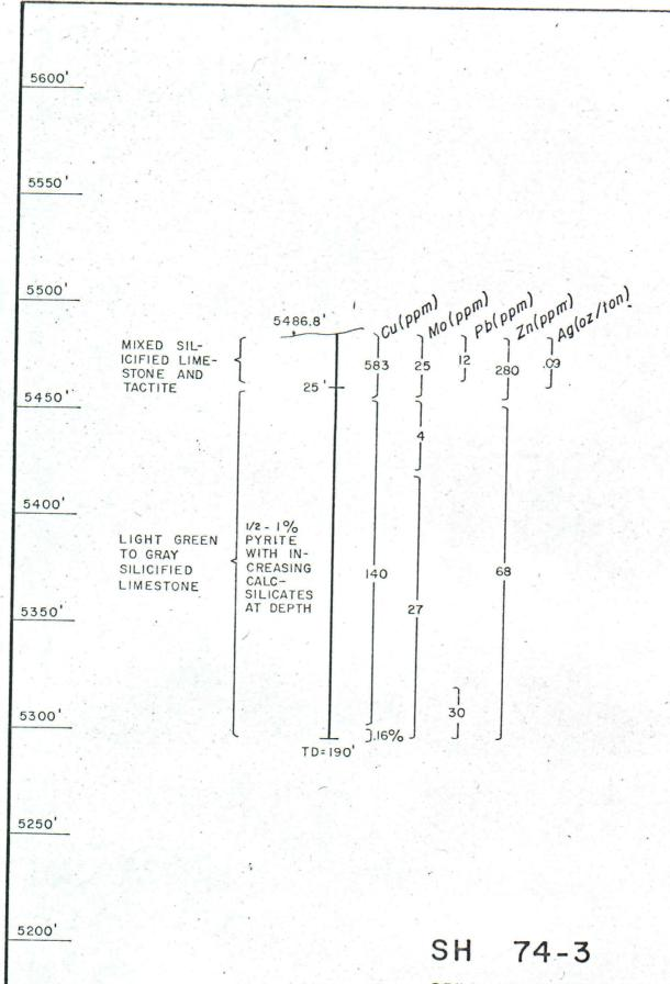
DRILL HOLE CROSS SECTION
