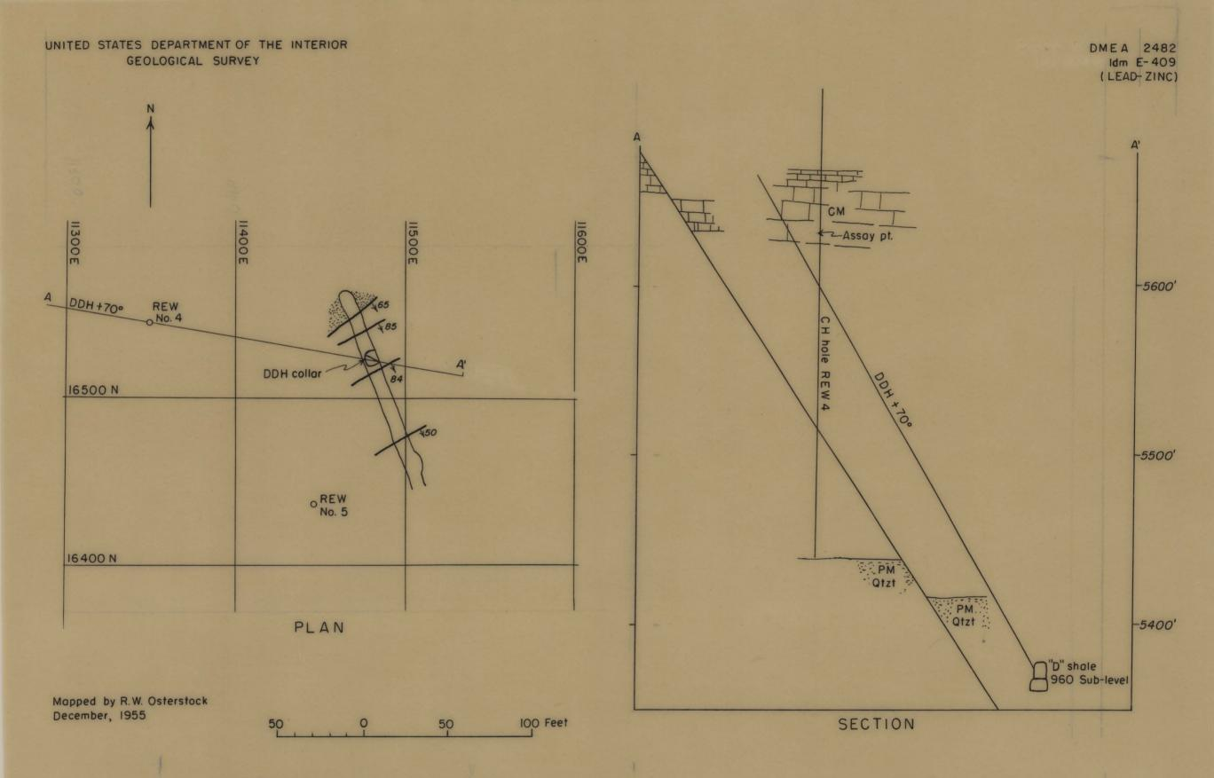
PLAN AND SECTION OF DIAMOND DRILL HOLE AREA NEAR FACE OF 960 SUB-LEVEL DRIFT
