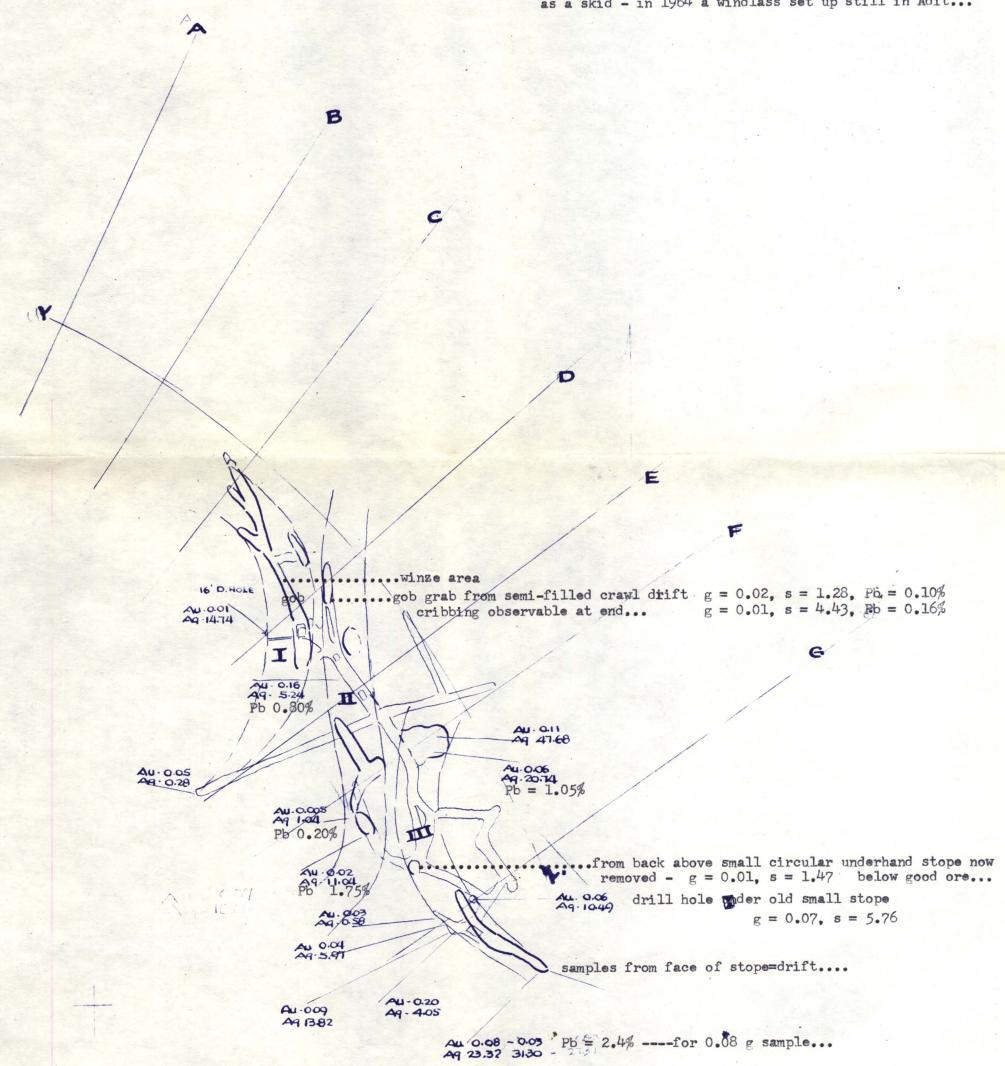
200' level.....with new workings off the new shaft at a slightly higher level than the old workings and an inadequate connection between the two
