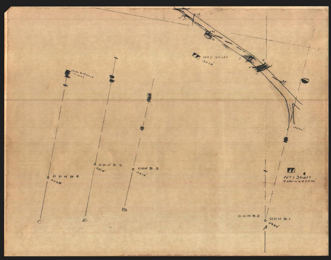
BUCKSKIN MINE DOUGLAS COUNTY, NEV. - PLAN-ADIT LEVEL -IINCH = 4-OFEET Diorite Monzonite Quartzite Minin (Feox, Oty, Cu-corb. ansulph) M.M. H. 4-63 Shaped up, rathru'to surfece
