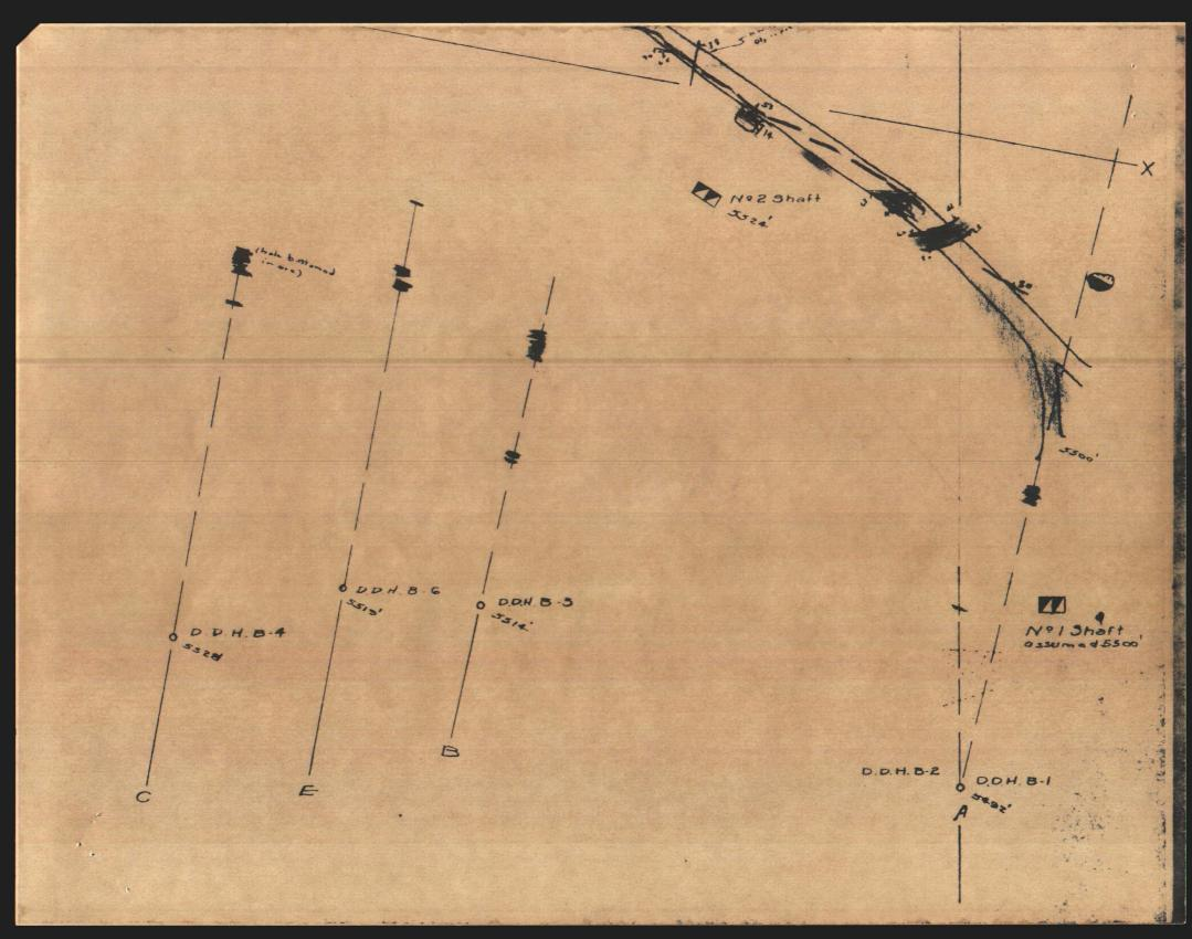
BUCKSKIN MINE DOUGLAS COUNTY, Nev. - PLAN-ADIT LEVEL -INCH = 40 FEET Diarite Monzonite Quartzite Minin (Feox, Ots, Cu-corb. ansulph) M.M. H. 4.63
