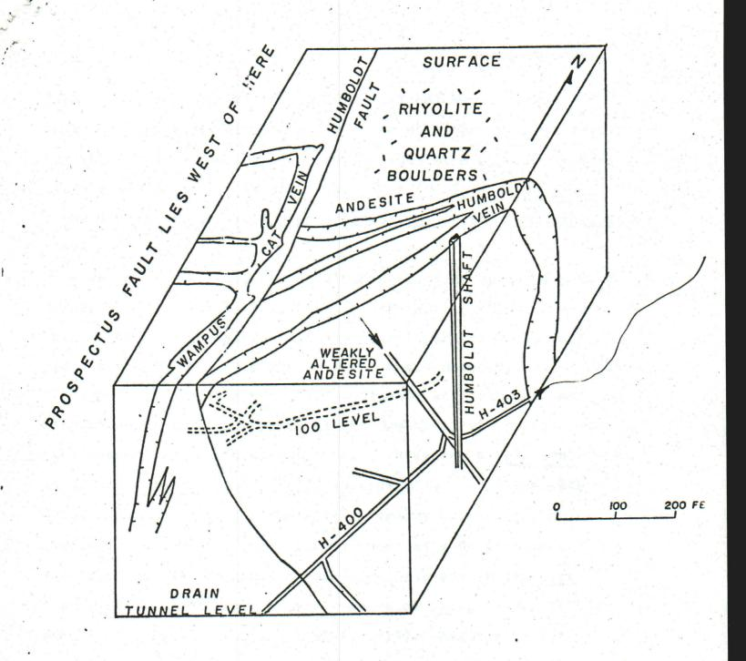
FIGURE 2 ISOMETRIC PROJECTION OF THE CENTRAL SECTION OF THE HUMBOLDT VEIN, HUMBOLDT HILL STOPING NOT SHOWN AREA WEST OF THE SHAFT IS NOW A GLORY HOLE MODIFIED BY L.P.JAMES FROM H.N. WITT 1915.
