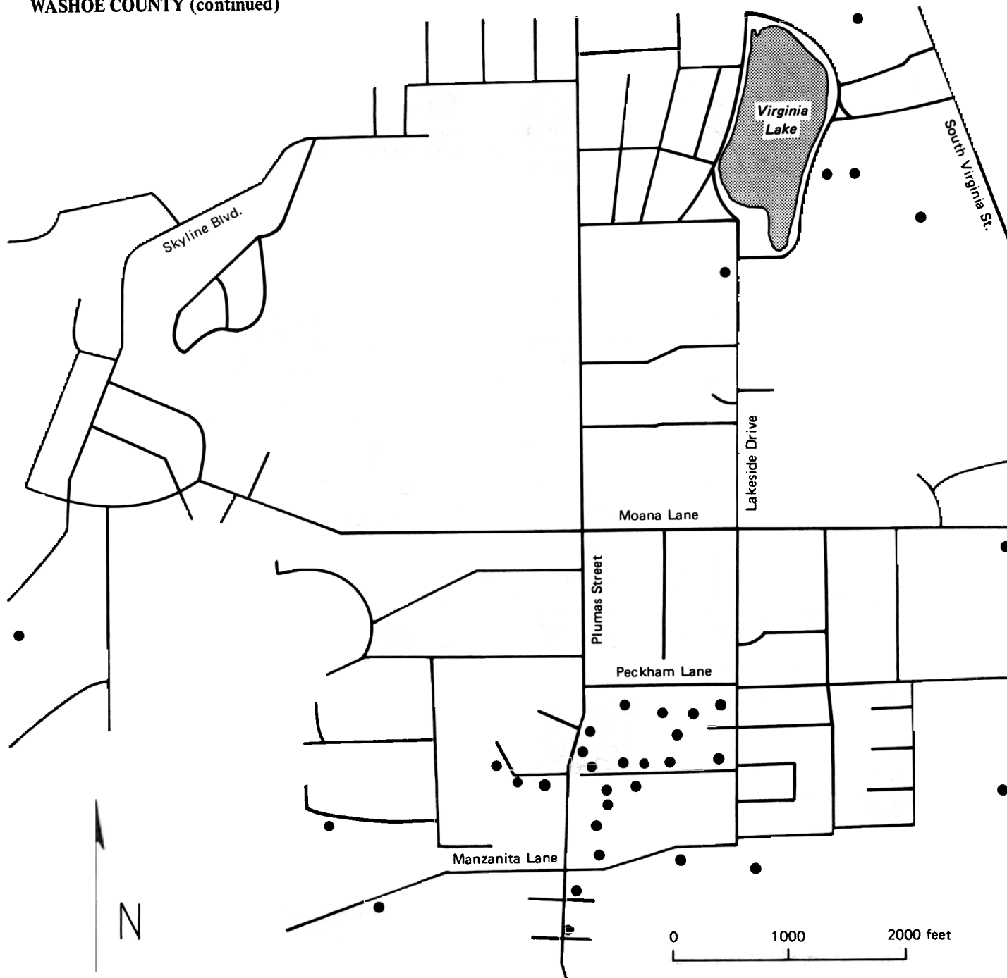
FIGURE 45. Map showing locations of shallow thermal wells in southwest Reno that are used for space heating, domestic hot water, and swimming pools (from unpublished map by R. B. Scheibach, 1974).
